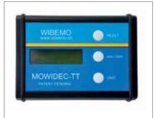
It couldn't be any simpler: the screen shows the error with the diameter to the nearest micron, then simply correcting the offsets compensates for the error. Recentring spindles becomes child's play!
