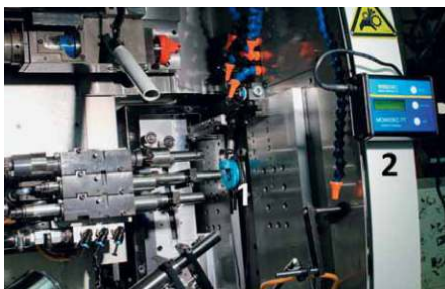
Mowidec-TT installed on a Tornos Deco 10 machine: 1) the sensor-bearing ring and 2) the control unit. The cable which connects the sensor to the unit can withstand the atmosphere in the machining area without any problems.
