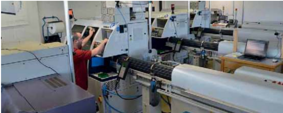
Within the Deco 10 workshop, the machines work 18 hours a day and 6 days a week in a controlled atmosphere. Tolerances of +/- 2 µ are commonplace.
