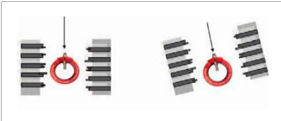
Fitting on the guide bush. The vertical axis of the sensor must be positioned along the same plane as the vertical axis moving the plattens.
