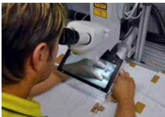
The jaw parts of the forceps are connected via joints with a draw piece. This is welded here by laser with a wire under magnification.
